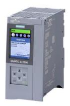
SIMATIC S7-1500F, CPU 1516F-3 PN/DP, central processing unit with work memory 3 MB for program and 7.5 MB for data 1st interface: PROFINET IRT with 2-port switch, 2nd interface: PROFINET RT, 3rd interface: PROFIBUS, 6 ns bit performance, SIMATIC Memory Card required \*\*\*\*approvals and certificates according to entry 109817466 at support.industry.siemens.com to be considered! \*\*\*\*
