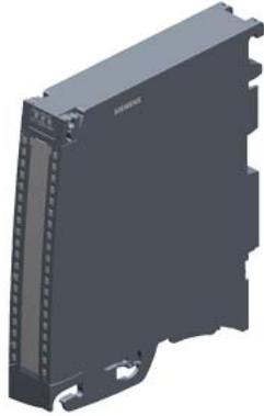
SIMATIC S7-1500 Analog input module AI 4xU/I/RTD/TC ST, 16 bit resolution, Accuracy 0.3%, 4 channels in groups of 4; 2 channels for RTD measurement; Common mode voltage 10 V; Diagnostics; Hardware interrupts; Delivery including push-in front connector, infeed element, shield bracket, and shield terminal
