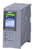
SIMATIC S7-1500F, CPU 1515F-2 PN, central processing unit with 1.5 MB work memory for program and 4.5 MB for data, 1st interface: PROFINET IRT with 2-port switch, 2nd interface: PROFINET RT, 6 ns bit performance, SIMATIC Memory Card required \*\*\* approvals and certificates according to entry 109817466 at to be considered! \*\*\*
