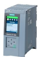
SIMATIC S7-1500, CPU 1515-2 PN, central processing unit with work memory 1 MB for program and 4.5 MB for data, 1st interface: PROFINET IRT with 2-port switch, 2nd interface: PROFINET RT, 6 ns bit performance, SIMATIC Memory Card required \*\*\* approvals and certificates according to entry 109817466 at support.industry.siemens.com to be considered! \*\*\*
