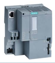
SIMATIC DP, CPU 1510SP-1 PN for ET 200SP, Central processing unit with Work memory 100 KB for program and 750 KB for data, 1st interface: PROFINET IRT with 3-port switch, 72 ns bit performance, SIMATIC Memory Card required, BusAdapter required for Port 1 and 2
