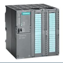
SIMATIC S7-300, CPU 314C-2PN/DP Compact CPU with 192 KB work memory, 24 DI/16 DO, 4 AI, 2 AO, 1 Pt100, 4 high-speed counters (60 kHz), 1st interface MPI/DP 12 Mbit/s, 2nd interface Ethernet PROFINET, with 2-port switch, Integr. power supply 24 V DC, Front connector (2x 40-pole) and Micro Memory Card required
